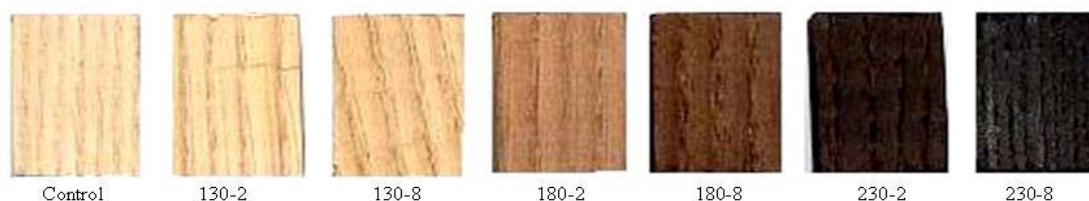
Figure 1. Color change with increasing heat treatment temperature and time
